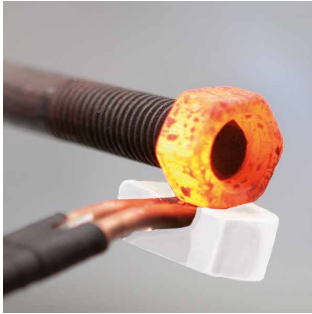
Releasing of rusted bolts
