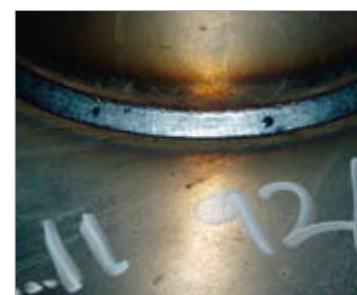
OK Tubrod 14.11-1.2mm in 92%Ar/% CO 2 -Torch angle 20° pushing. Pipe to plate connection.
