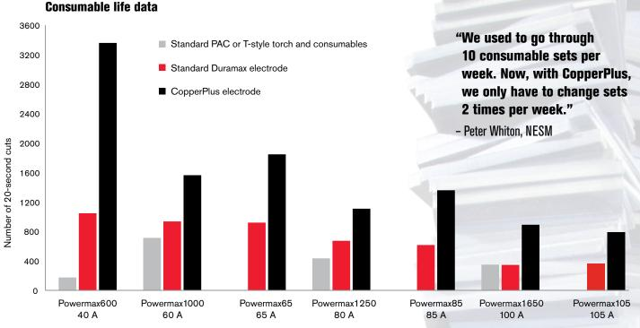
Note: Lab testing shows that CopperPlus will deliver at least 2 times longer consumable life in most cases; consumable life may vary depending on the system, amperage and process.
