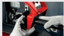
/The Fronius System Connector serves as a central connection-point for all media. It lets users lock the hosepack simply and safely, with no tools, to ensure a quaranteed defined current transfer.
