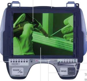
The "tack welding comfort mode" uses an intermediate light state (shade 5). If a follow-up arc is not struck within two seconds, the welding lens switches to the normal light state (shade 3). The comfort mode helps reduce eye fatigue resulting from the eye constantly needing to adjust to differing light levels during tack welding.
