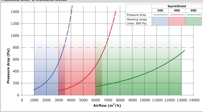
The installation of any product(s) not included in the initial design of an extraction system could add additional static pressure to the overall system design. By doing so, the result may be a reduction of airflow at the extraction point.
