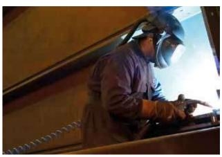
Supplied air solutions are ideal where welding gases may build up displacing breathing air.
