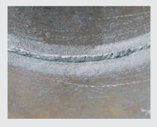
/ Superb results are also achieved when welding pipelines with Cel electrodes. The optimised properties of the arc prevent the electrode from breaking or sticking. The result – a 100% homogeneous root.
