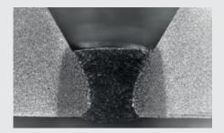
/ The LSC Root characteristic even impresses on challenging root passes with a perfect root formation and penetration.
