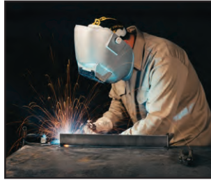
Conventional CV short circuit transfer, using carbon dioxide (CO2) and .045 in. solid wire.
