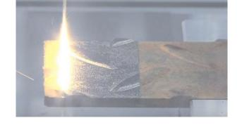
By using a laser cleaning machine you can remove dirt, oxides, coatings, paints, oils and many more. This technology is fast and environmentally friendly. Laser cleaning technology works in such a way that a beam generated by a laser source communicates through a fiber optic cable to a system of mirrors that transmit the laser in the desired shape and configuration. In the head there is a Galvo system which is the instrument that conducts the laser beam in one direction or another.
