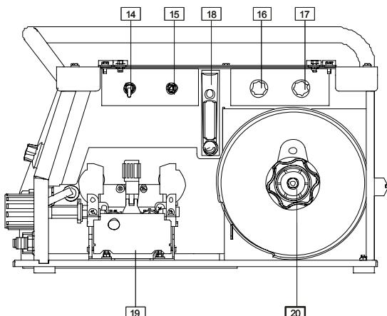
14. Torch Mode Switch: It enables selection of 2-step or 4-step torch mode. The functionality of 2T/4T mode is shown in the picture below:
