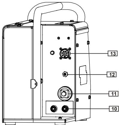
10. Quick Connect Couplings: If water cooled torches are used, connect water lines from water cooler here. Refer to torch and water cooler guidelines for recommended cooling liquid and flow rates.
