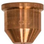
**The nozzle** is the most frequently replaced consumable. One of the signs that the nozzle needs to be changed is an excessive amount of both dross and bevel angle appearing in your cuts. On the nozzle itself, you will find that a larger orifice or an irregularly shaped hole will be the telltale signs of excessive wear.
