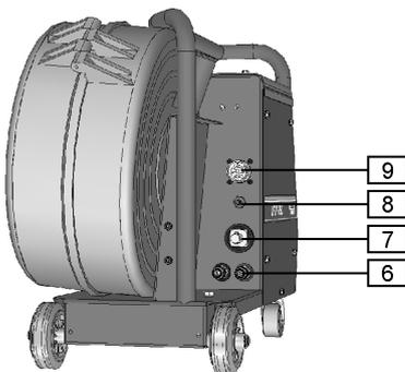
6. Quick Connect Couplings (For water cooled model only): If water cooled torches are used, connect
