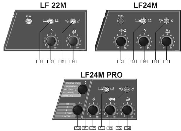
10. Wire Diameter Knob: It allows the choice of the wire diameter requested for the desired welding process. This feature is available only for the synergic mode.
