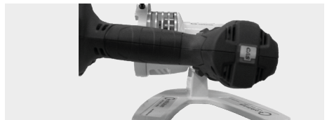
Electric variant (RPG 3.0): Set the switch in the center position to block the On/Off switch
