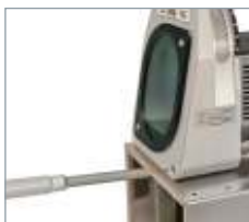
Precise adjustment of the electrode's stick-out.
