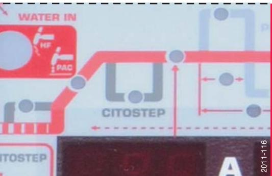
With the CITOSTEP function available on ADVANCED version, two current levels can be chosen, the welding current and the basic current. This facilitates the change from one to the other by rapidly pressing the torch trigger. The CITOSTEP function can be used to adjust heat input momentarily, to change welding positions or to replenish the filler metal supply without having to stop welding.
